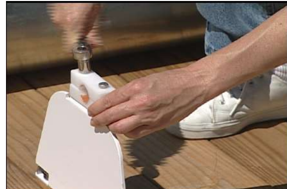
Tighten only to a snug fit, making sure the drum can still turn freely.
