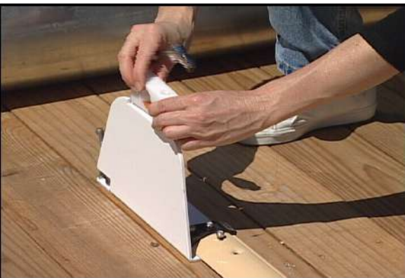
Using a 7/16 socket or wrench, loosen the two bolts to remove the top half of the white delrin shaft retaining blocks. Follow this procedure for the opposite side.
