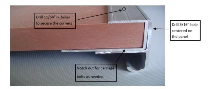
You will also want to secure the corners down. Using an 11/64'in bit drill a hole through the top of the "B2" extrusion, 2"in. from the end and 1/2" from the front edge. The hole should go through the "B2" extrusion, panel and the horizontal edge of the "L2" extrusion. Follow up with a counter sink bit. Insert and secure a 1 3/4" stainless steel screw. Repeat for the other side.
